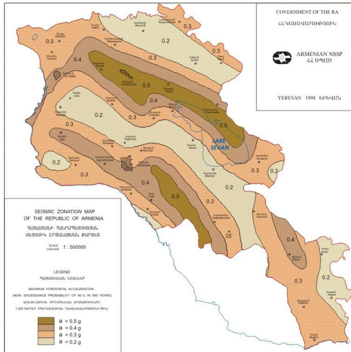
**Figure 1.** The long-term seismic hazard map of the territory of Armenia, compiled by the Armenian NSSP in 1998.
